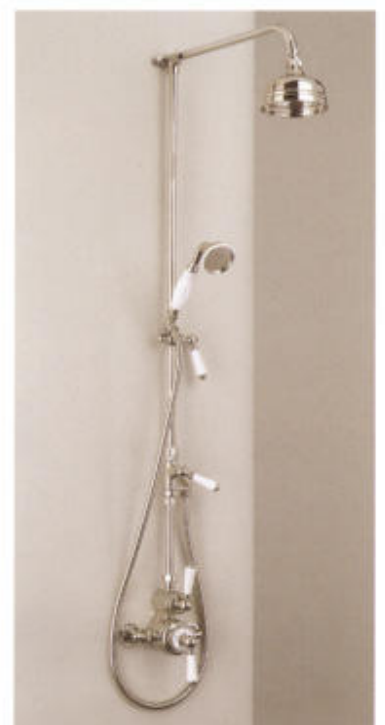
Exposed thermostatic valve with 18mm overhead shower arm with 5" skirted shower rose, riser, diverter valve & handshower on riser rail.
